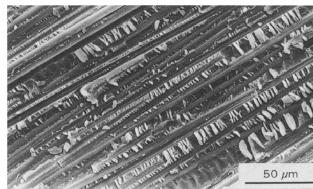
Figure 11 Mode II fracture surface of BASF Material D with unstable crack growth.
